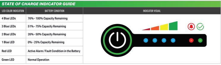
The Trojan® GC2 36V Lithium-Ion features include a battery status push button and indicator light on the top of the case. A momentary press of the button displays the battery's State of Charge and operating status.
